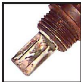
Ethylene Glycol (Antifreeze) Contamination
